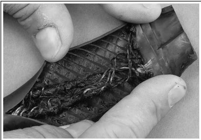
Damaged Fuel Hose
