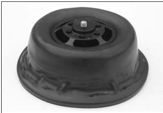
Damaged Fuel Pump Diaphragm
