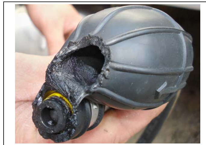
Deteriorated fuel hose and primer bulb
