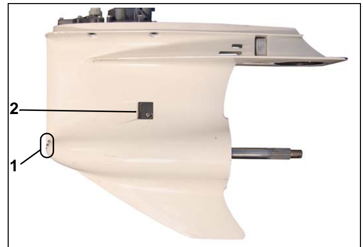
M2-Type Gearcase 1. Front water inlet 2. Side water inlet
