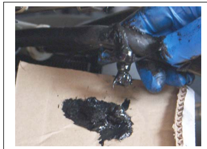
Blockage in the fuel system
