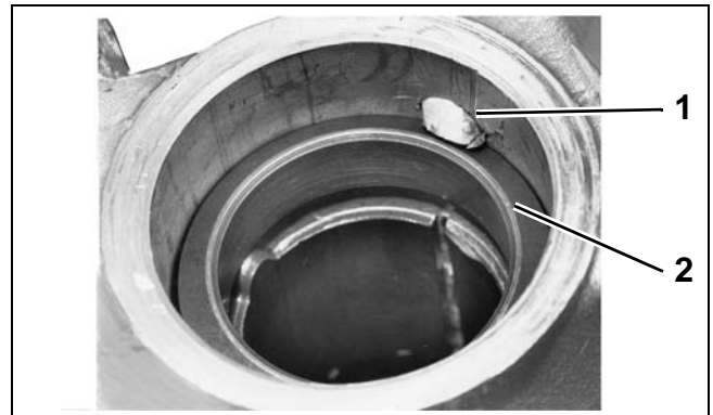
1. Steering friction pin 2. Steering friction thrust ring COA2988
