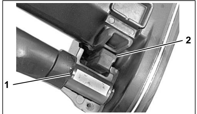
1. Thrust washer 2. Lower front mount
