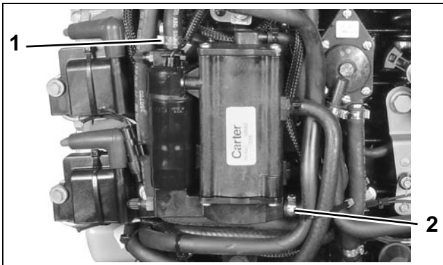
1. Fuel supply manifold 2. Fuel return manifold
