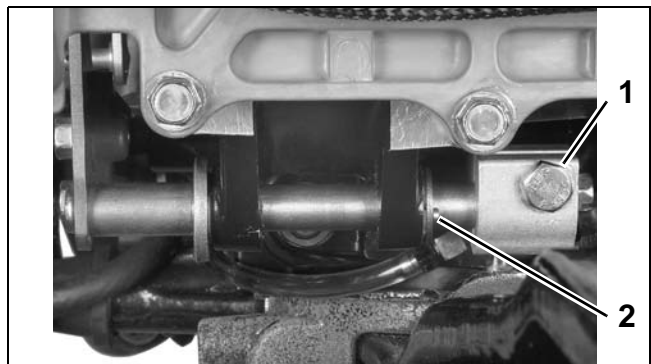
1. Shift rod lever screw 2. Cotter pin
