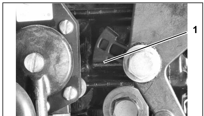
1. Throttle lever stop – 2 Cylinder models 005114
