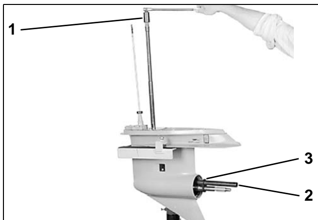
1. Holding socket 2. Pinion holder 3. Retainer 42229
