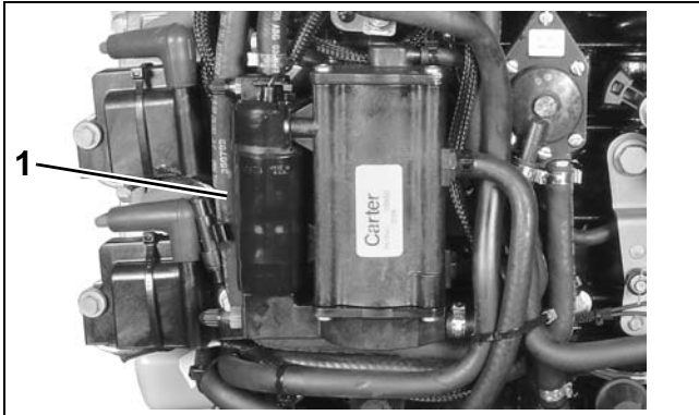
Vapor Separator Assembly 1. Circulation pump
