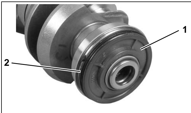
1. Lower seal housing 2. O-ring
