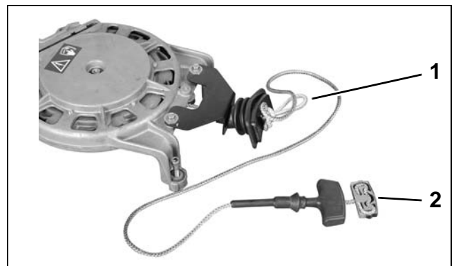
1. Slip knot 2. Rope anchor 007853
