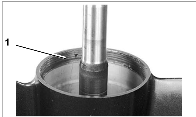
1. Hydrostatic seal grooves
