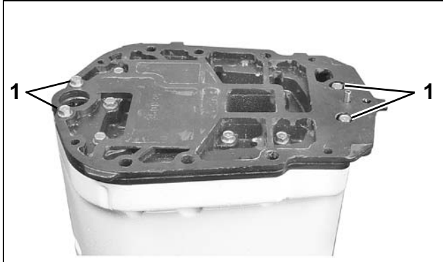
1. Adapter retaining screws 001981
