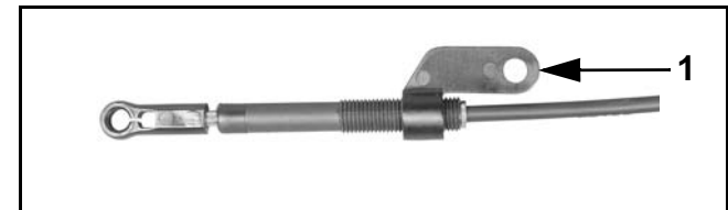
1. Turn anchor four turns toward cable end.
