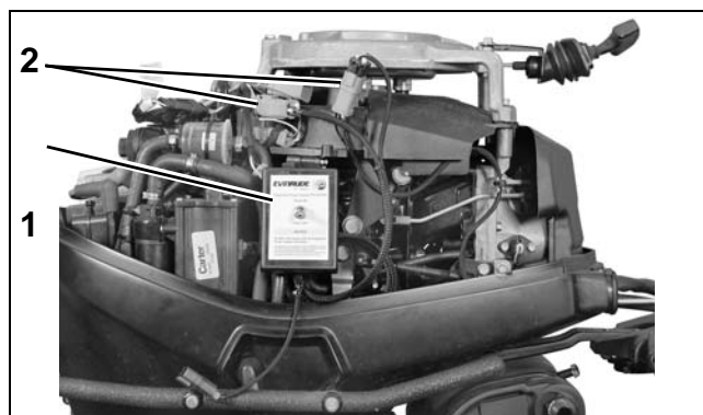
1. Power supply tool 007279 2. Engine harness connectors
