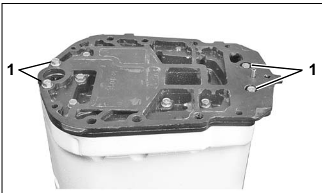
1. Adapter retaining screws
