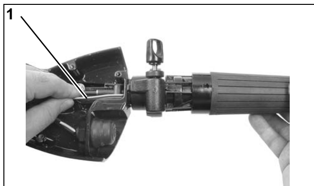
1. Trim switch wiring 006677
