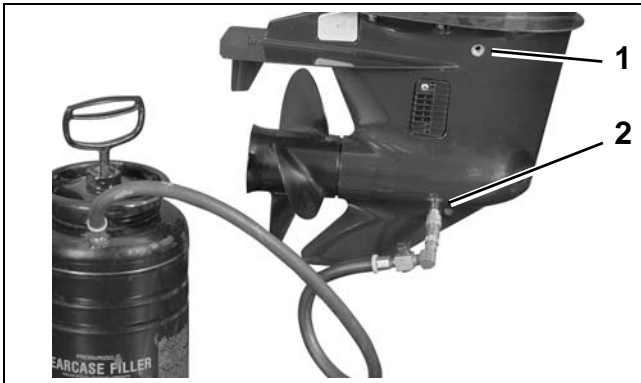
1. Lubricant level plug 2. Lubricant drain/fill plug
