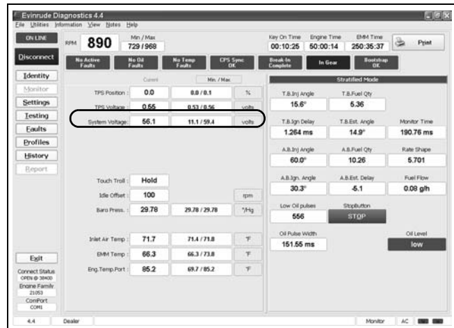
Monitor Screen, System voltage
