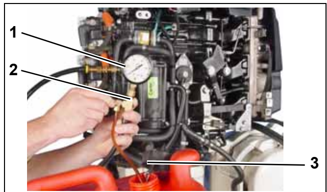
1. Test fitting 2. Venting valve 3. Venting hose
