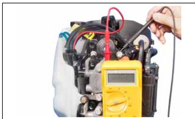
1. Oil injection pump connector (pin 2) 008065
