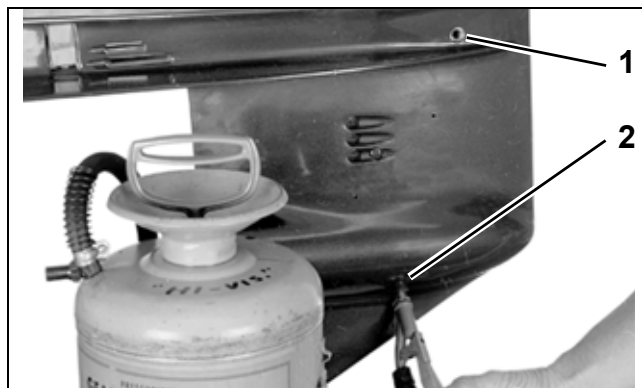
1. Lubricant level plug 2. Lubricant drain/fill plug
