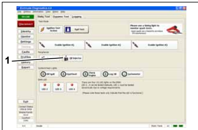
Static Tests Screen 008082A 1. Oil injector test button
