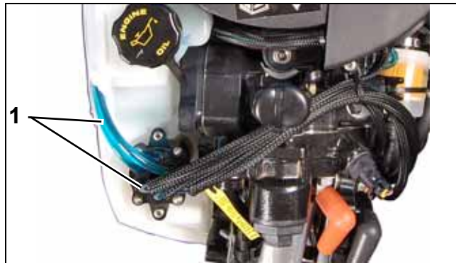
1. Oil distribution hoses
