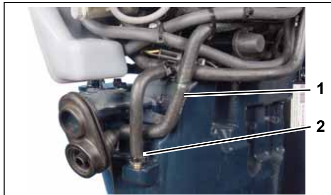
1. Overboard indicator hose 2. Drain hose
