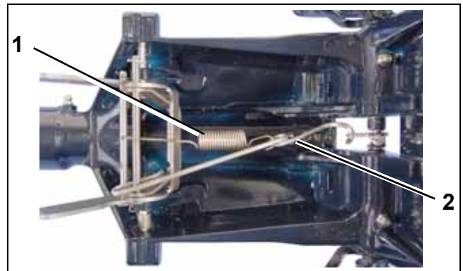
1. Spring 007615 2. Reverse lock release rod
