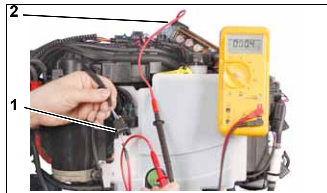
1. Oil injection pump connector pin A 2. EMM connector pin 2 007328
