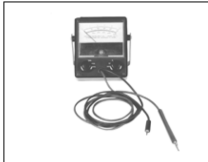
Peak reading voltmeter 49799 P/N 507972
