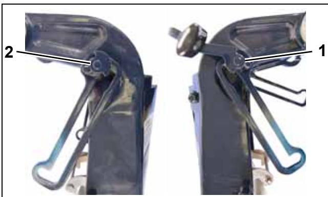
1. Port stop link cam 007611 2. Tilt lock lever cam 007612
