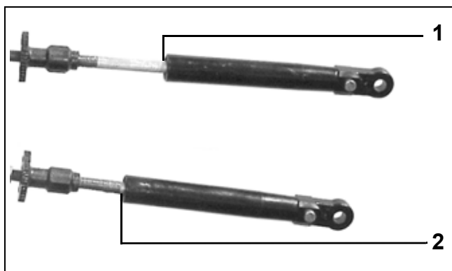
1. Shift cable casing guide extended to midpoint 2. Throttle cable casing guide retracted DP0811
