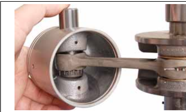
1. Gap of retaining ring 2. Notch in piston
