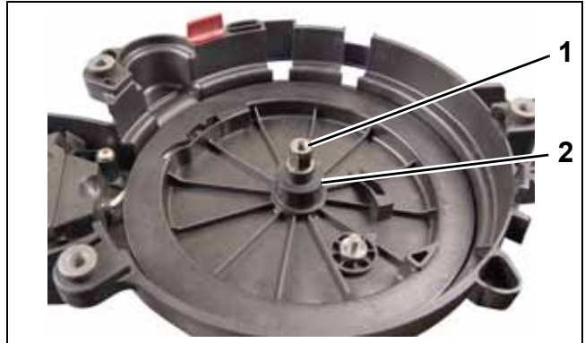
1. Left-hand threaded nut 2. Retainer 007727
