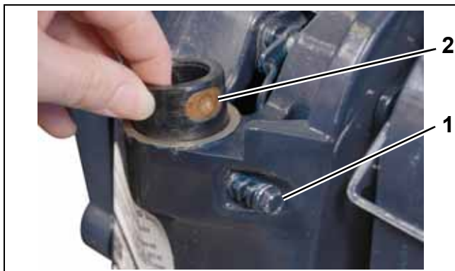
1. Friction plate 2. Friction screw
