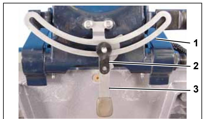
1. Steering friction plate 2. Steering friction washers 3. Steering friction lever
