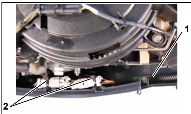
1. Wire routing 007125 2. Secure with two tie straps
