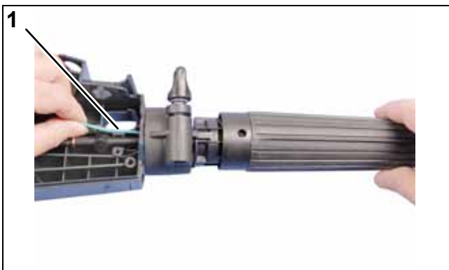
1. Trim switch wiring
