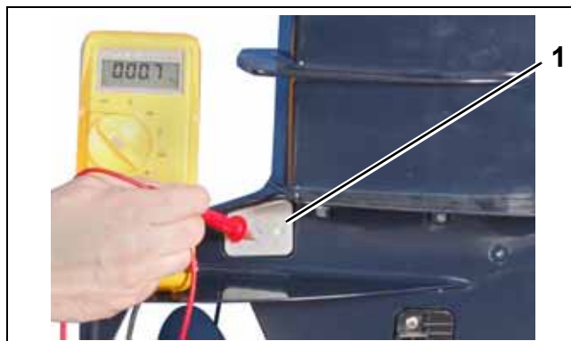
1. Meter lead to anode 007268
