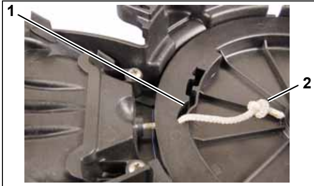
1. Rope channel 2. Knot 007709
