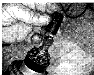
Fig. 128 The typical snapping retained drive unit used on some models utilizes a protective cap...
