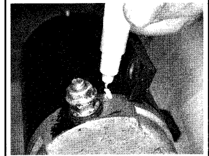
Fig. 133 If not already done, matchmark the end caps (commutator and drive) to the starter housing for assembly purposes
