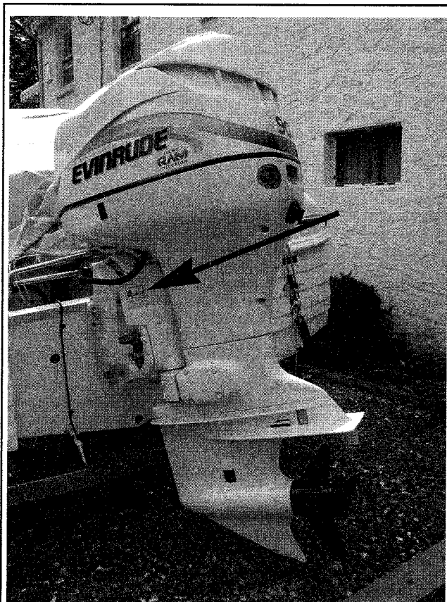
Fig. 1 A model ID tag and an emission control label are found on the port side of most engine transom/swivel/tilt brackets
