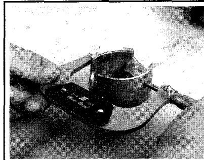
Fig. 85 Measure the piston outer diameter using a micrometer
