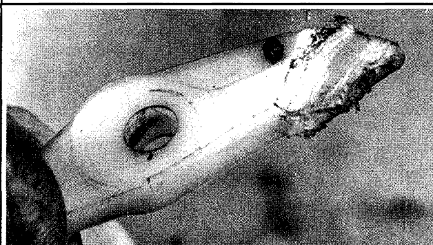
Fig. 19 Inspect the pawl for wear or damage (this one must be replaced)
