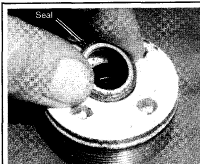
Fig. 76 Inserting the seal into the trim cylinder cap.
