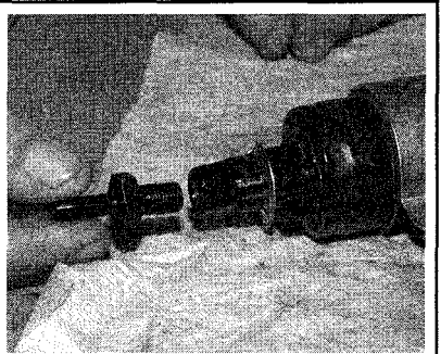
Fig. 202 Top fining unthreaded from the pump
