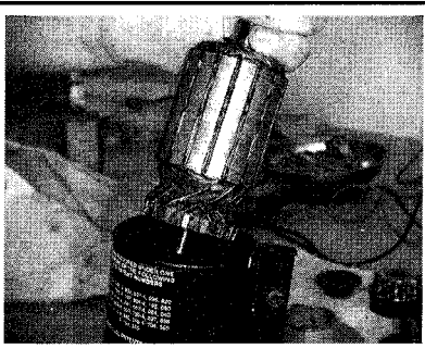
Fig. 138 Take care when inserting the armature in the starter housing, as permanent magnets will pull it inward strongly
