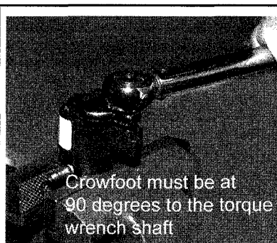
Fig. 59 Then tighten using crowfoot adapter and torque wrench
