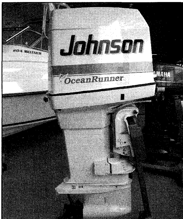
Fig. 16 The powerhead alone for V8 motors can weigh more than 370 lbs. (161 kg)...
