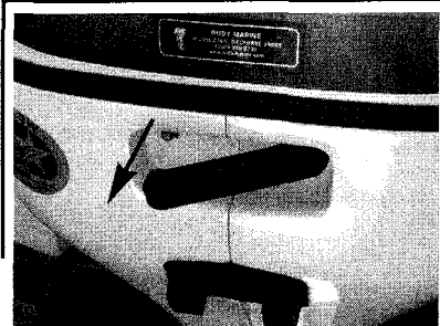
Fig. 33 Release top cover latches by pulling outward on one end...
