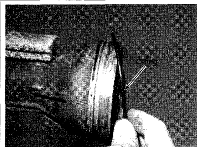
Fig. 42 Slide or cut the O-ring(s) off the bearing carrier (number and location vary, so note them for installation purposes)
