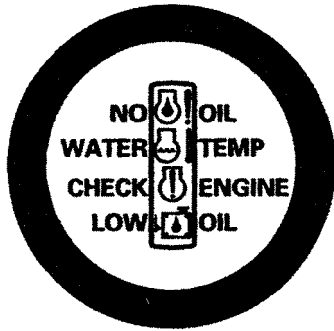
Fig. 176 The System Check monitor in normally installed in the boat dash as a stand-alone gauge...
