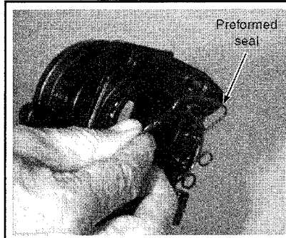
Fig. 93 Install a new preformed seal in the groove on the carb body
