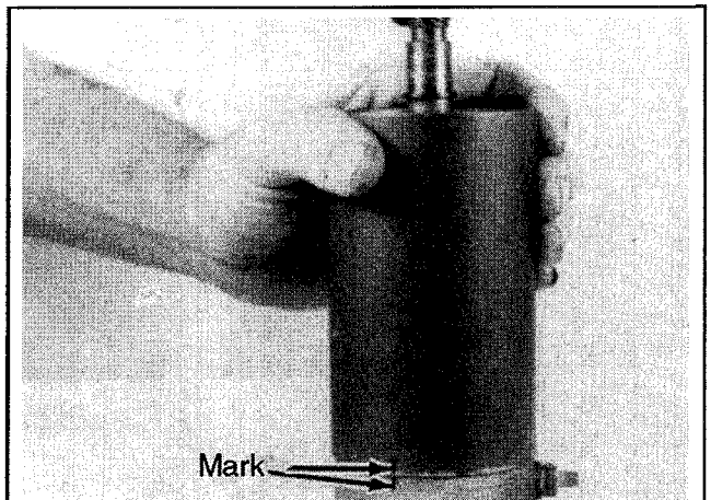
Fig. 143 Align the matchmarks as the housing is placed in position
