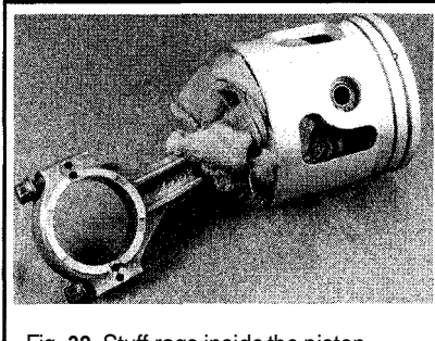
Fig. 32 Stuff rags inside the piston skirt to protect it from damage by the connecting rods anytime the rod is removed from the crankshaft journal
