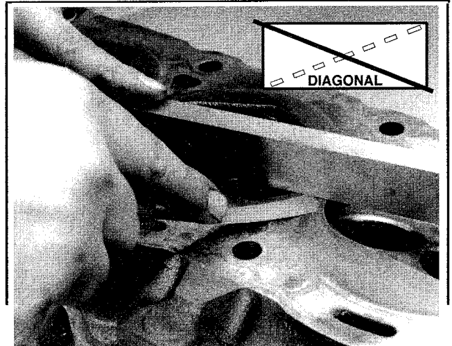
Fig. 70 ... and at diagonals across the head to be sure the surface is within specification for reuse
