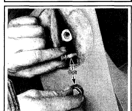
Fig. 16 Remove the 2 gearcase bolts threaded upward under the ventilation plate (location varies)
