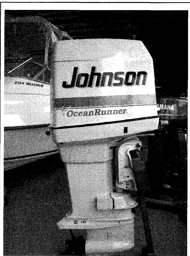
Fig. 41 The lower cover screws are normally found on the starboard side of V6 engines, or the port side of V4 and V8 motors
