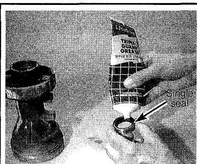
Fig. 112 Coat all seal lips with marine grade grease
