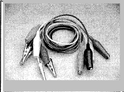
Fig. 5 Jumper wires are simple, but valuable pieces of test equipment
