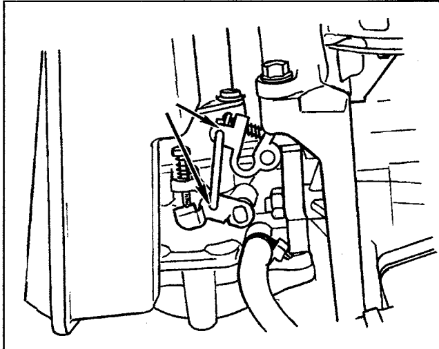
Fig. 25 Carburetor linkage lubrication - 51618 hp (164cc) motors (4 Deluxe similar)
