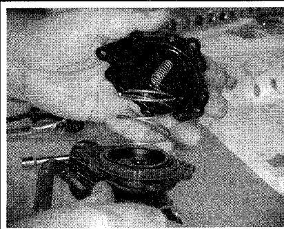
Fig. 17 Remove the air motor cover slowly, carefully releasing the spring pressure
