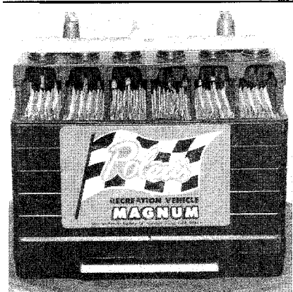
Fig. 132 A fully charged battery, filled to the proper level with electrolyte, is the heart of the ignition and electrical systems. Engine cranking and efficient performance of electrical items depend on a full rated battery
