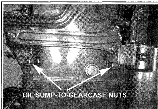
Fig. 19 Remove the oil sump-to-gearcase nuts to free the powerhead and sump assembly
