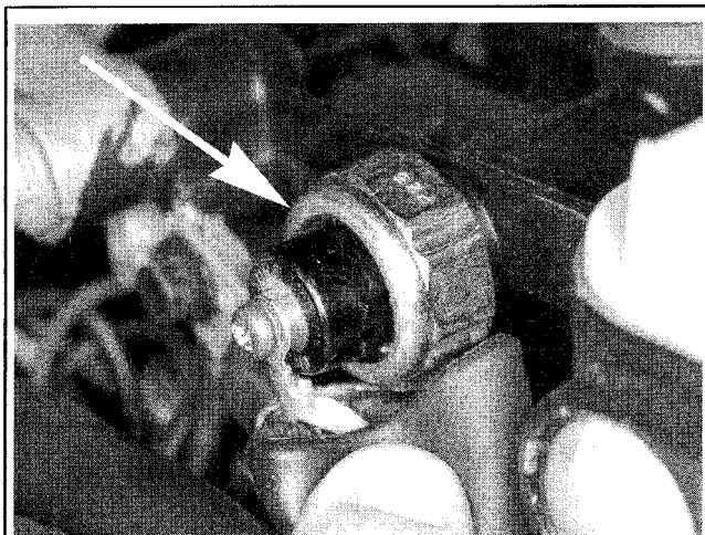
Fig. 237 Although oil pressure switch location varies slightly by model, it is always threaded into an oil passage on the powerhead
