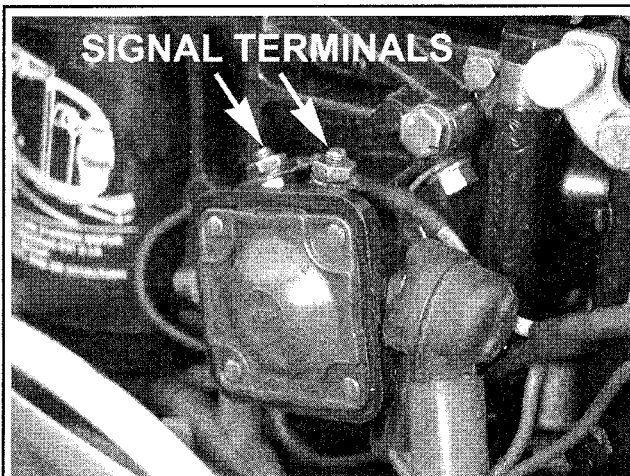
Fig. 230 Typical Johnson/Evinrude starter solenoid with signal terminal identification - used on most 2-strokes, 4-stroke models similar but vary in terminal
