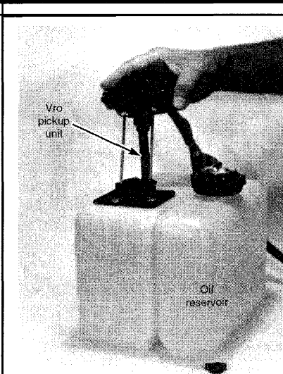
Fig. 6 If necessary for testing or inspection, the oil tank pickup unit is easily removed from the tank. . .
