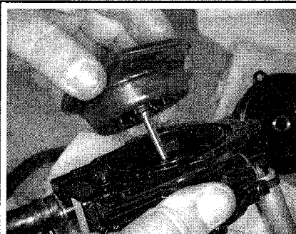
Fig. 24 Once the air motor and fuel pistons/diaphragms are compressed and unthreaded, carefully pull the air motor diaphragm (with the piston stem in this case) from the intermediate housing. . .
