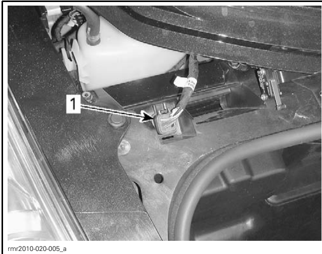
1. Communication connector stored in protective cap
