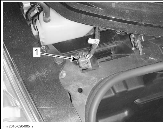
TYPICAL 1. Vehicle communication connector location
