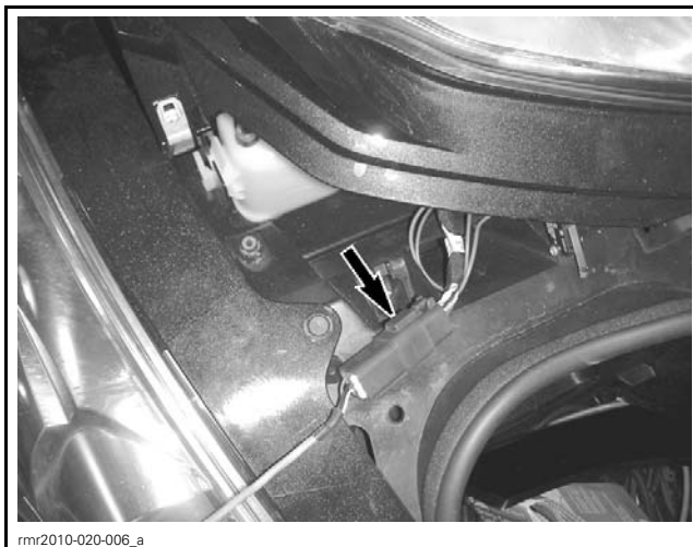
TYPICAL - MPI-2 CONNECTION TO VEHICLE COMMUNICATION CONNECTOR
