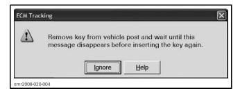
When this occurs, turn the ignition key OFF and wait until the message disappears (approximately 20 seconds after key removal).
