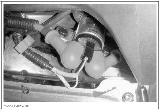
STARTER SOLENOID (RH FUEL TANK COVER REMOVED)
