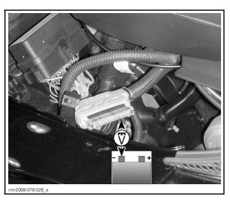
If voltage is not good, check wiring/connectors between TCM and main relay 2. Refer to *WIRING DIAGRAM*.
