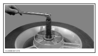
Using the BLIND HOLE BEARING PULLER SET (P/N 529 036 117), remove and discard wheel bearing.
