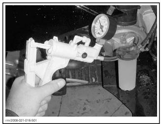
ACTIVATE PUMP UNTIL FLUID REACHES CLUTCH RESERVOIR
