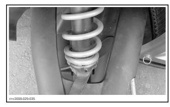
Turn the adjusting cams clockwise to increase spring preload.
