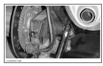
Loosen rear axle tensioner screws. Be careful not to unscrew tensioner screws completely.
