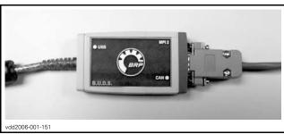
Connect the MPI-2 USB connector to the USB port on the PC (personal computer).
