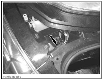
TYPICAL - MPI-2 CONNECTION TO VEHICLE COMMUNICATION CONNECTOR
