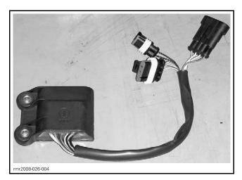
The D.E.S.S. module is located behind the front frame member.
