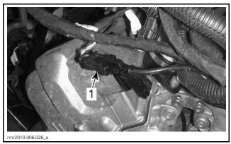
1. Crankshaft position sensor (CPS)
