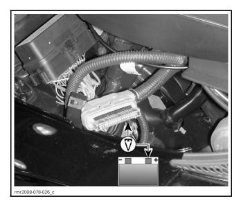
If ground circuits are not good, check wiring and connections between TCM and battery ground.
