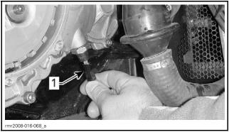
1. Oil pressure switch connector
