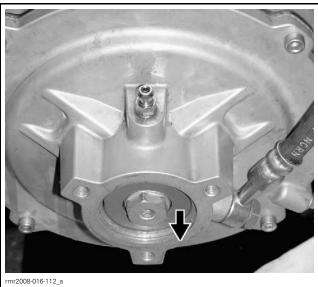
MOVEMENT OF CLUTCH HYDRAULIC PISTON
