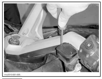
**NOTICE** Leave cover on reservoir to avoid spillage during the following procedure.
