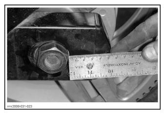
Tighten rear adjuster screws to same length on both sides of swing arm.
