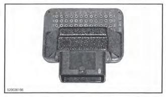
Using a multimeter set to "Ω", test for continuity between the oxygen sensor harness connector and the ECM adaptor as per following tables.
