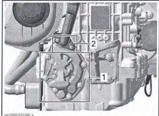
1. Screws M6 x 25 2. Screws stainless steel M6 x 45
