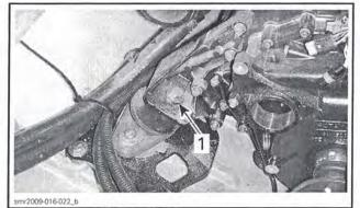
TYPICAL - LEFT SIDE OF VEHICLE 1. Rear engine support screw
