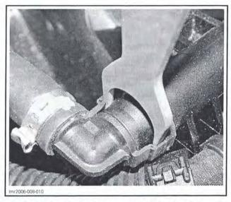
**NOTE:** It may be necessary to rotate fuel hose fitting to align the tool ends with the openings of the locking mechanism.
