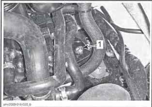
TYPICAL - RIGHT SIDE OF VEHICLE 1. Rear engine support screw
