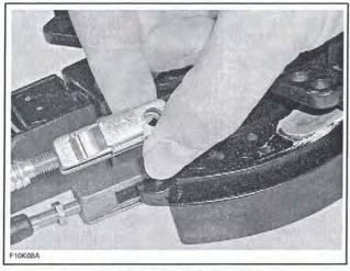
REMOVE CABLE CONNECTOR FROM SHIFTER
