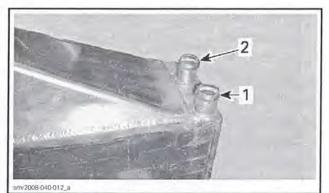
Intercooler water inlet fitting Intercooler water outlet fitting 1.
