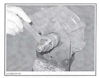
Check slipping moment counterclockwise by using a torque wrench with a viewer.
