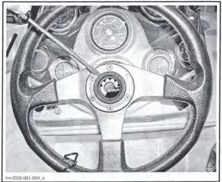
TYPICAL — CAREFULLY REMOVE WITH A SMALL SCREWDRIVER
