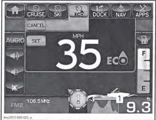
COMPASS BUTTON BLINKS YELLOW WHEN FAULT OCCURS 1. Fault icon
