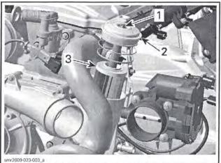
TYPICAL – 210 CHALLENGER SHOWN 1. Oil filter screw 2. Oil filter cover 3. Oil filter
