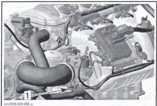
1503 SUPERCHARGED INTERCOOLED ENGINE 1. Throttle position sensor (TPS)
