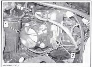
**TYPICAL** - **ETA** 1. Throttle body 2. Throttle actuator
