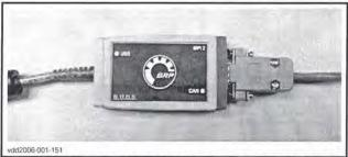
DIAGNOSTIC CABLE CONNECTED TO MPI-2 INTERFACE CARD
