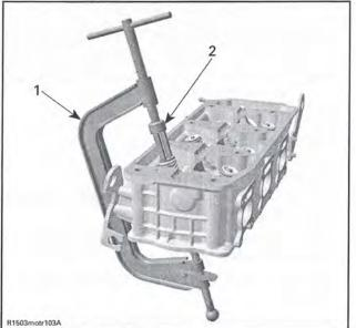
. Valve spring compressor clamp
