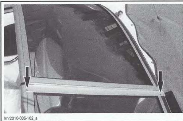
Imr2010-035-102_a RETAINING RIVETS
