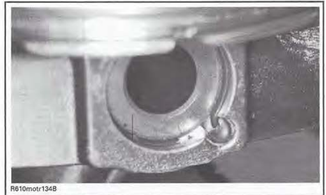
CORRECT POSITION OF THE PISTON CIRCLIP
