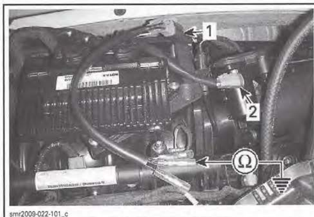
smr2009-022-101_c STATOR INSULATION TEST 1. Connect adapter to magneto connector 2. Leave vehicle harness disconnected
