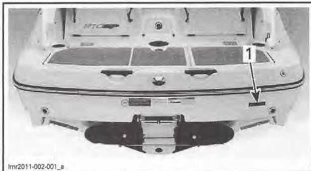
TYPICAL 1. Hull Identification Number (H.I.N.)
