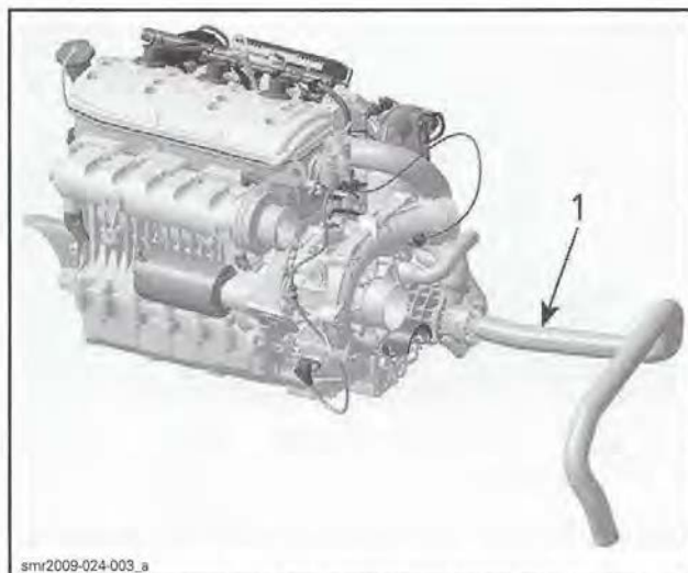
1. This hose becomes hot when thermostat opens
