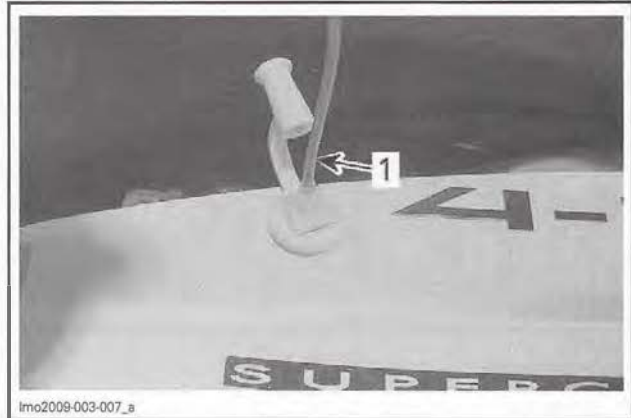
TYPICAL 1. Can needle into lubrication fitting
