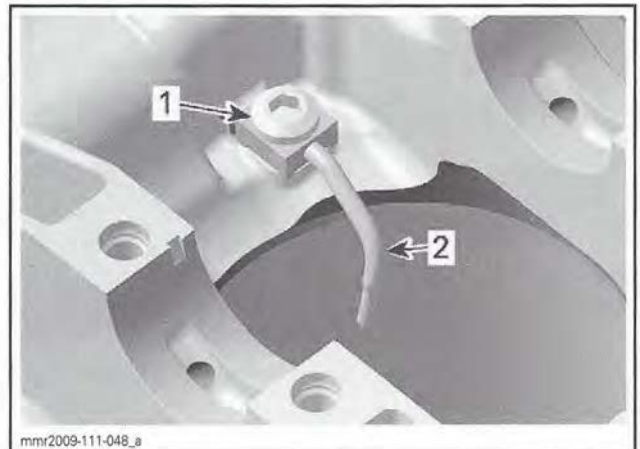
mnr2009-111-048_a 1. Banjo fitting 2. Oil spray nozzle
