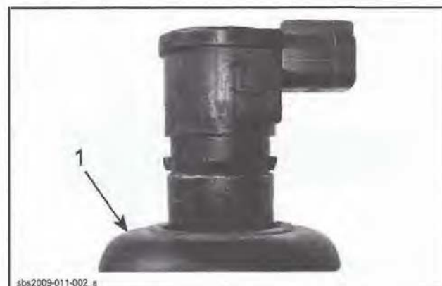
1. Rubber seal pulled down
