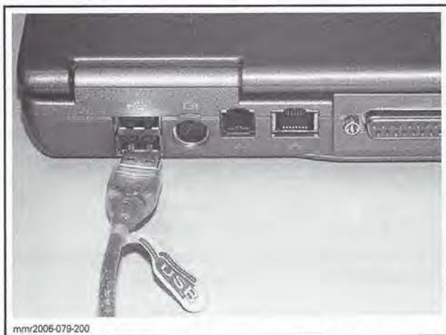
MPI-2 INTERFACE CARD CONNECTED TO USB PORT
