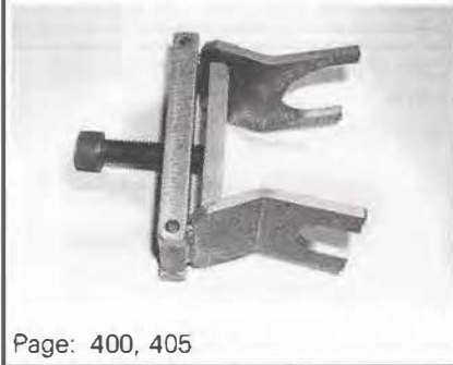
FLOATING RING TOOL (TYPE III) (P/N 529 035 987)
