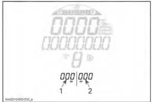
lmo2010-003-030_a HOURLY METER 1. Port side 2. Starboard side
