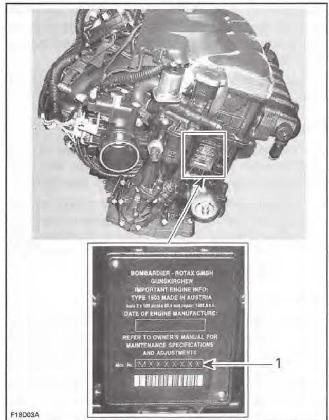
1. Engine Identification Number (E.I.N.)
