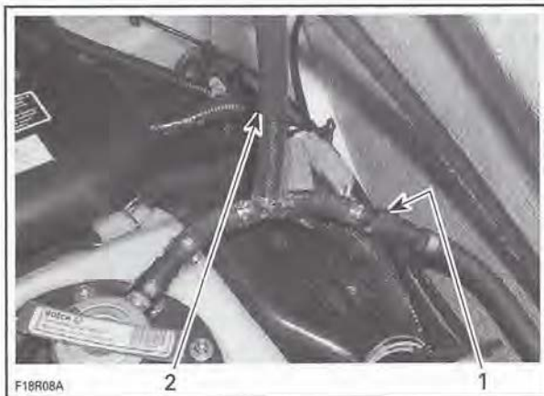
TYPICAL 1. Hose disconnected from fuel pump 2. In-line installation of fuel pressure gauge
