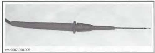
BACK PROBE INSTALLED ON MULTIMETER PROBE
