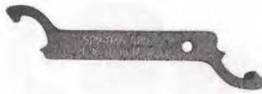
SUPERCHARGER GEAR HOLDER (P/N 529 036 025)
