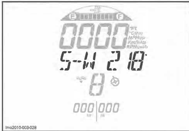
lmo2010-003-028 MULTIFUNCTION DISPLAY - COMPASS HEADING INDICATED
