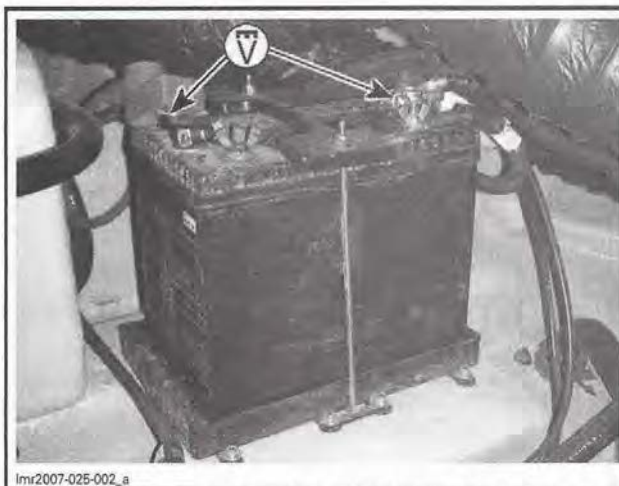
lmr2007-025-002_a TYPICAL - CHARGING SYSTEM VOLTAGE TEST AT BATTERY POSTS
