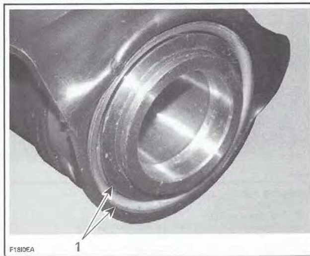
CORRECT POSITION 1. Inner sleeve flush with outer circumference
