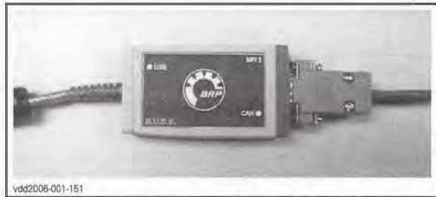
DIAGNOSTIC CABLE CONNECTED TO MPI-2 INTERFACE CARD
