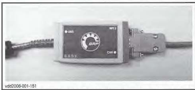
D.E.S.S. POST INTERFACE CONNECTED TO MPI-2 INTERFACE CARD
