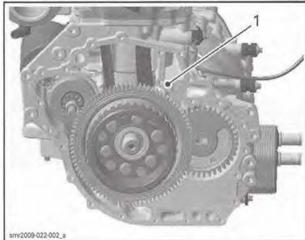
TYPICAL 1. Pay attention that gasket remains properly positioned on this surface
