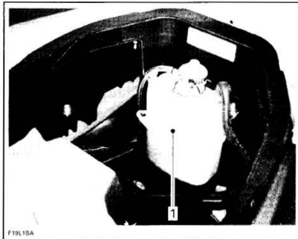
1. Coolant expansion tank
