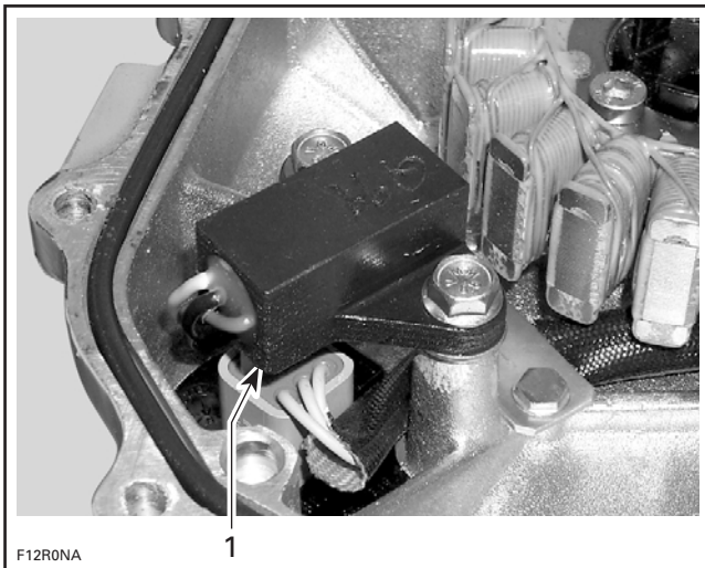
1. CPS inside magneto cover
