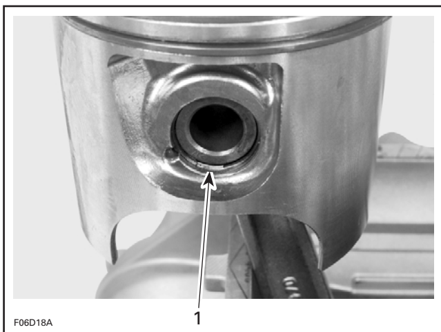
1. Circlip opening at 6 o'clock (at bottom)
