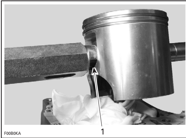
1. Tool cutout toward bottom of piston
