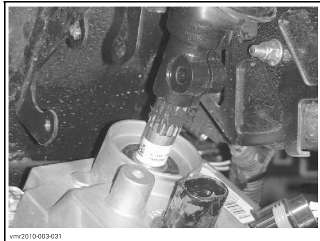
STEERING COLUMN INDEXED TO DPS SHAFT SPLINES
