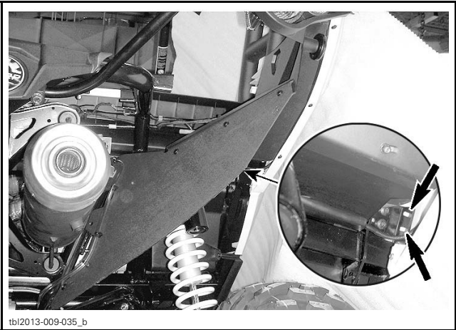
BESIDES SCREWS OF REAR CAGE ATTACHMENT POINT
