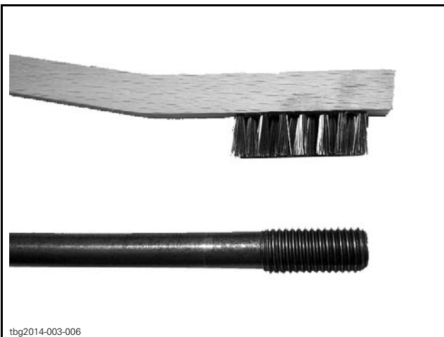
STUD END RECEIVING COUNTER NUTS
