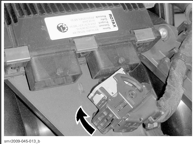
CONNECTOR LOCKING CAM IN RELEASE POSITION
