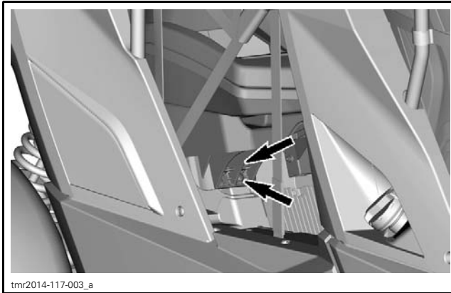
FRONT RETAINING SCREWS TO REMOVE
