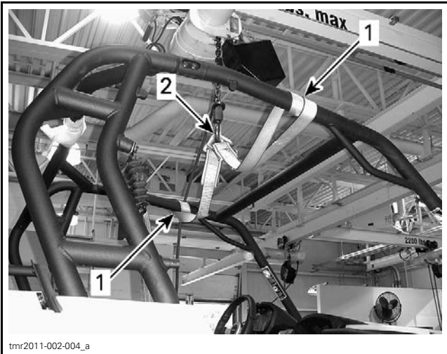
2-UP MODELS 1. Lifting strap around horizontal side tubes (top) 2. Hoist hook
