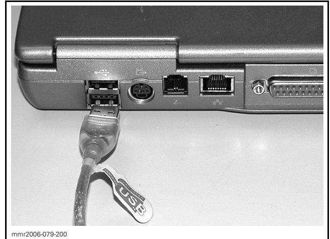
MPI CARD CABLE CONNECTED TO USB PORT
