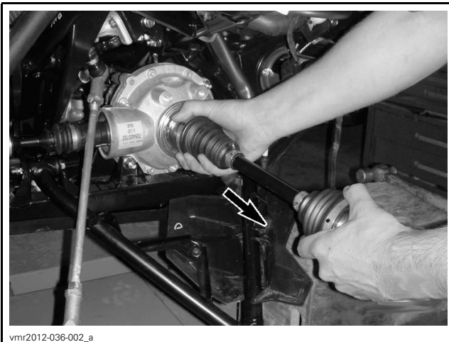
PULL DRIVE SHAFT
