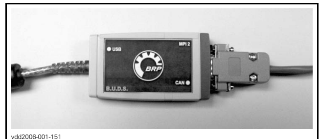
DIAGNOSTIC CABLE CONNECTED TO MPI-2 INTERFACE CARD
