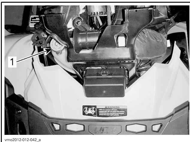
1. Cooling system pressure cap
