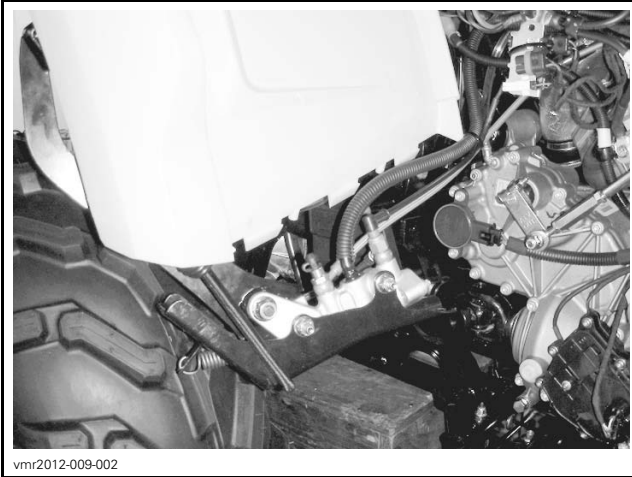
TYPICAL - MASTER CYLINDER SECURED TO REAR FENDER
