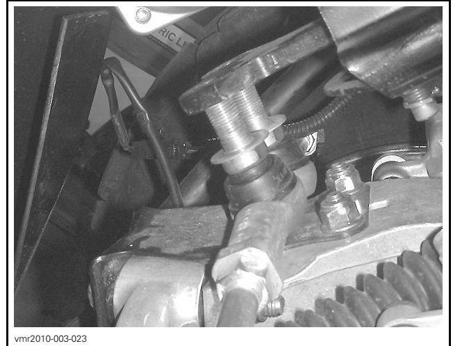
TYPICAL - TIE ROD ENDS (HARDWARE REMOVED)
