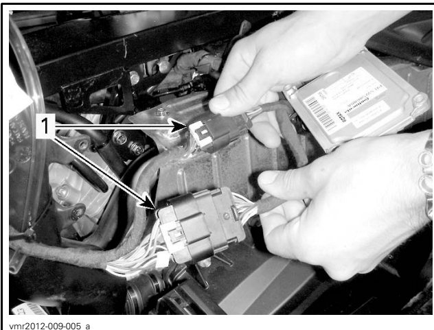
TYPICAL - LH SIDE OF VEHICLE 1. Engine harness connectors (HIC)
