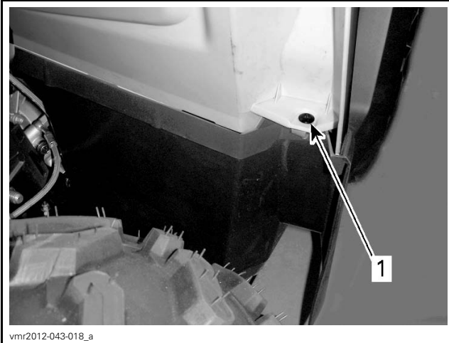
1. Screw securing rear fender
