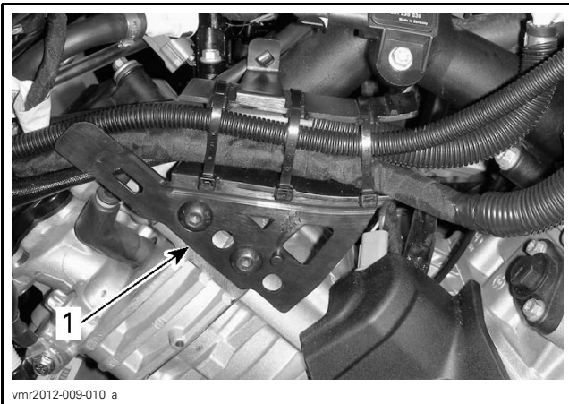
TYPICAL - RH SIDE OF ENGINE 1. Harnesses support
