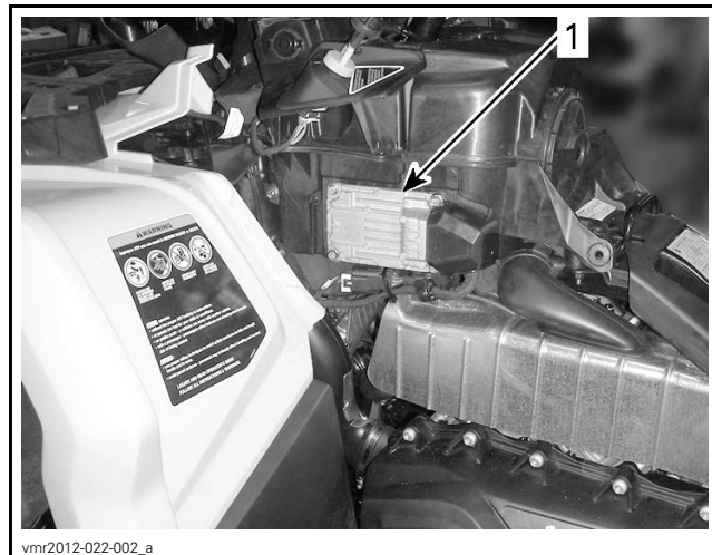
LH PANEL REMOVED 1. ECM location
