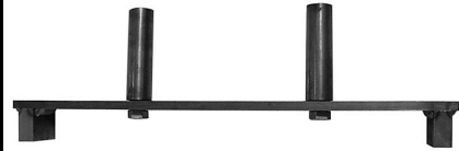
STEERING ALIGNMENT TOOL (P/N 529 036 059)
