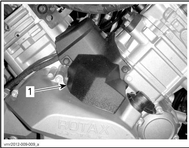
TYPICAL - RH SIDE OF ENGINE 1. Oil pressure switch cover
