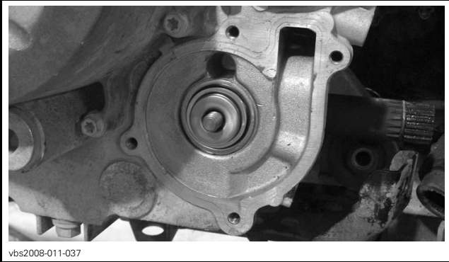
ROTARY SEAL PROPERLY SEATED ON CRANKCASE
