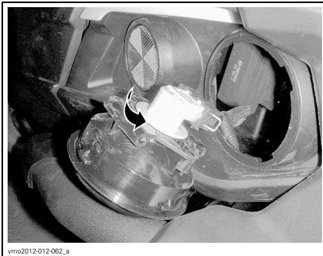
vmr2012-012-062_a ROTATE BULB COUNTERCLOCKWISE
