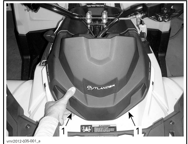
1. Push in and lift up here (both sides)
