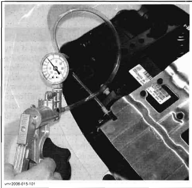
PUMP ON INLET SIDE
