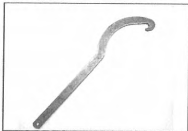
Drive pulley holder (CVT) P/N 529 006 400 Recommended
