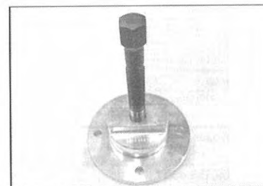
Hub puller P/N 529 035 612 Recommended
