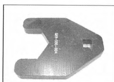
Crow foot P/N 529 035 884 Recommended Rally 200 Rear axle nut
