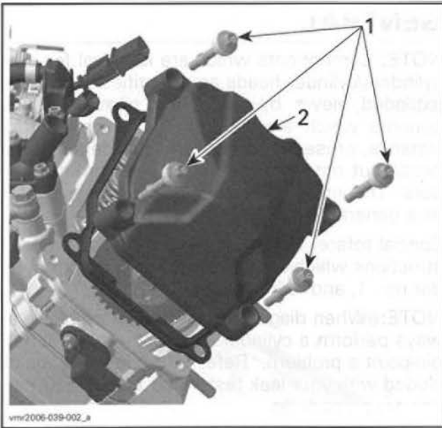
1. Distance screws 2. Valve cover
