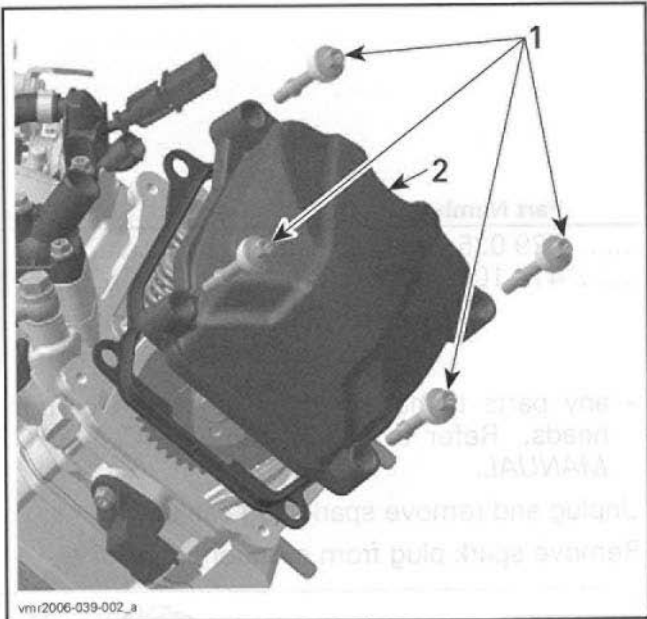
1. Valve cover screws 2. Valve cover
