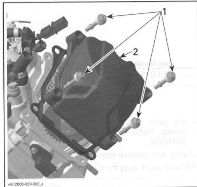
1. Valve cover screws 2. Valve cover
