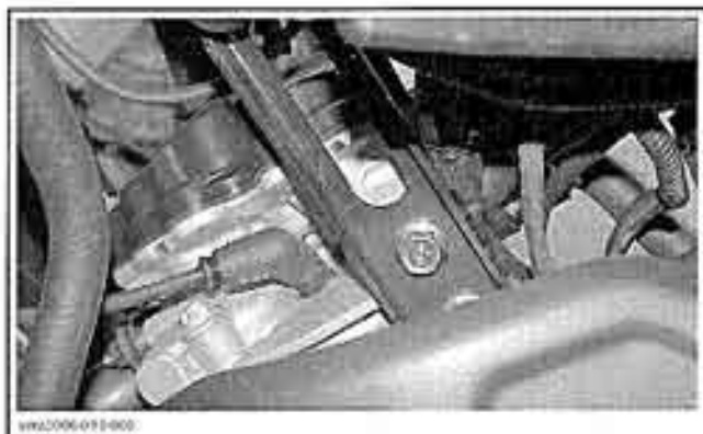
FRONT SPARK PLUG CABLE
