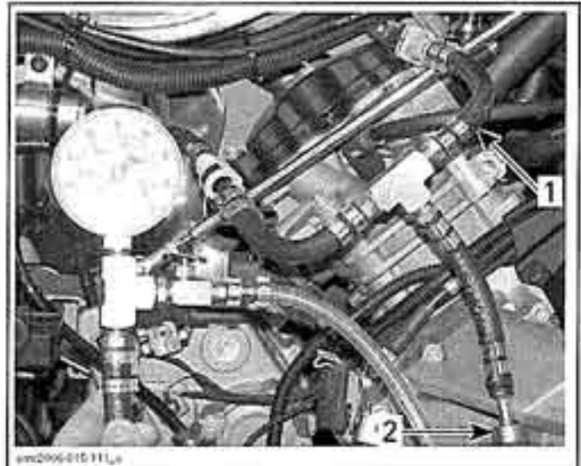
1. T-fitting — In-line installation 2. Fuel pressure gauge connection
