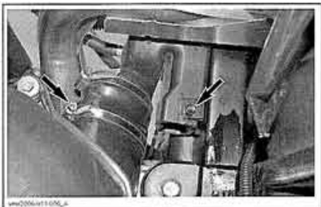
CVT OUTLET HOSE (UNSCREW BOTTOM CLAMP AND BOLT)
