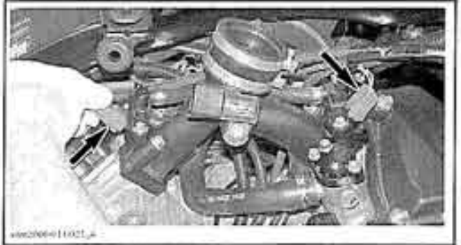
FUEL INJECTOR CONNECTORS
