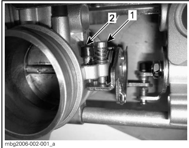
Unscrew idle speed screw [1] until the throttle body plate stop lever rests against its zero position stopper screw (capped screw) [2]. If necessary, loosen the throttle cable. Open throttle approximately one quarter then quickly release. Repeat 2-3 times to settle throttle plate.
