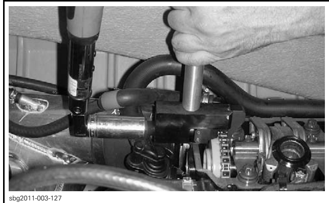
TIMING CHAIN MASTER LINK TIGHTENING
