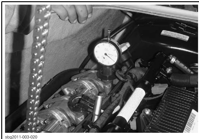
CYLINDER 3 POSITIONED AT TDC
