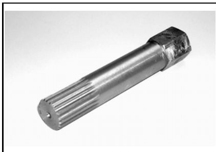
impeller remover/installer P/N 529 035 820 Mandatory 4-TEC 1503 NA and BV Also used to turn the engine.
