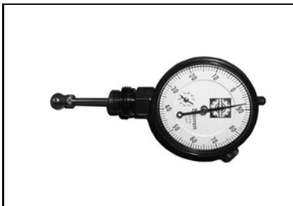
TDC Dial Indicator P/N 295 000 143 Recommended 2-stroke engines except DI, 1203
