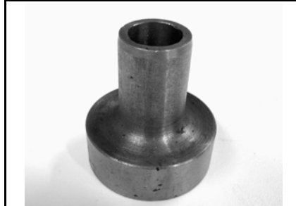
Pump Bearing Pusher P/N 529 035 818 Mandatory 4-TEC 1503 models
