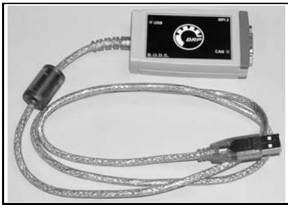
MPI-2 interface card P/N 529 036 018 Mandatory Replaces the MPI.
