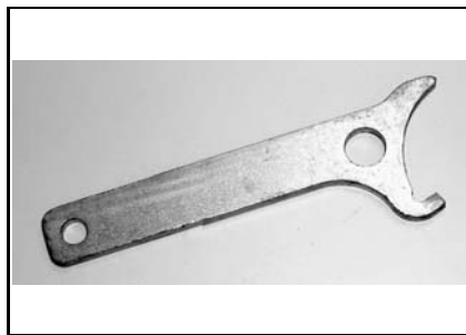
Shock preload adjustment wrench P/N 529 032 900 Recommended
