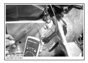
One extremity of the test wires has a small flat and slightly rounded shape to back probe various connectors. The other extremity fits our multi-meter test probe. These test wires are very useful to conduct resistance and voltage tests on connectors without damaging or disconnecting them.
