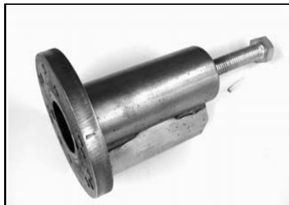
Crank shaft bearing puller P/N 529 036 004 Recommended 2 strokes Engine
