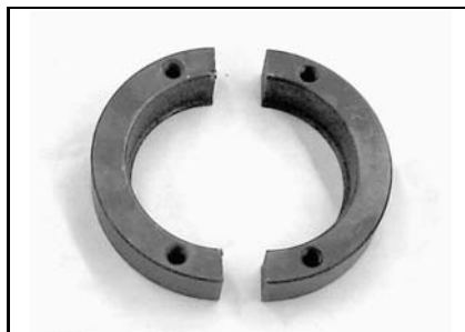
Half ring puller P/N 420 876 330 Recommended 947 & 947 DI engines To remove 52 mm O.D. bearings from the crankshaft.
