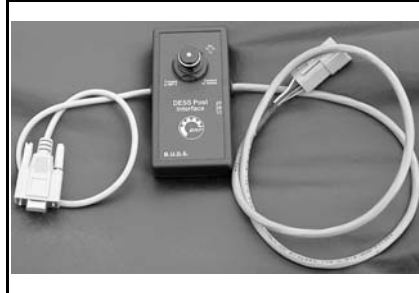
D.E.S.S. Post Interface P/N 529 036 019 Mandatory To programm D.E.S.S. keys with the MPI-2.
