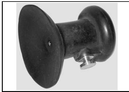
Suction Cup P/N 295 000 163 Recommended To remove gauges.
