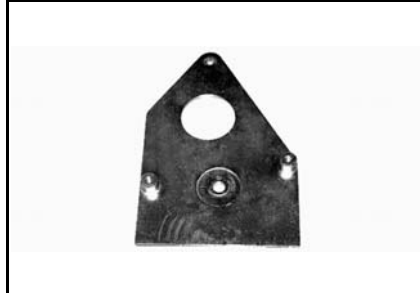
SUPPORT PLATE P/N 529 035 947 Mandatory 4-TEC 1503 SC To hold the supercharger assembly in a vise for disassembly and assembly.
