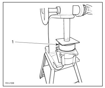
1. Install wear ring into jet pump housing as shown.
