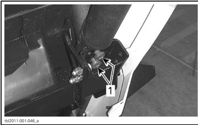
TYPICAL — RH REAR CAGE ATTACHMENT POINT 1. M10 x 30 TORX screws
