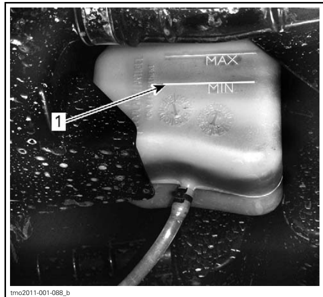
COOLANT EXPANSION TANK 1. MIN level
