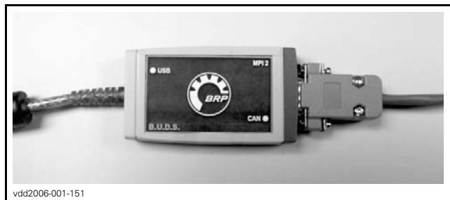
DIAGNOSTIC CABLE CONNECTED TO MPI-2 INTERFACE CARD
