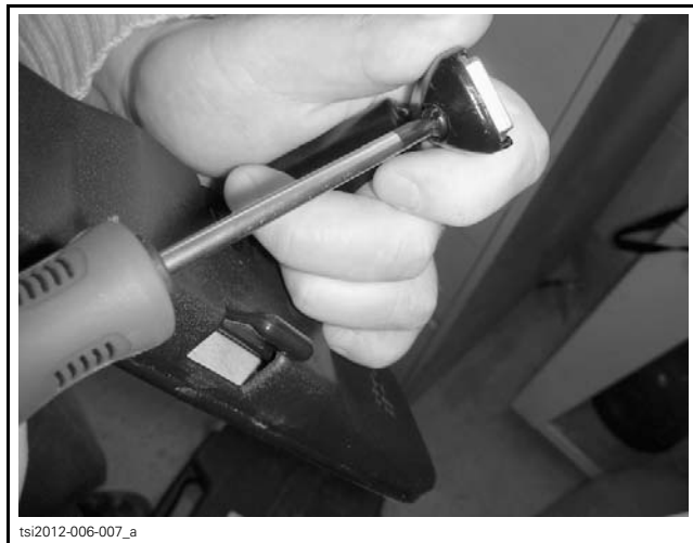
LOOSENING SCREW TO REMOVE THE METAL BUSHING
