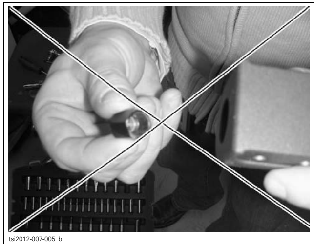
INCORRECT NUT ORIENTATION
