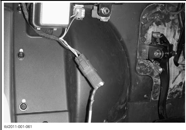
MPI-2 INTERFACE CARD CONNECTED TO USB PORT
