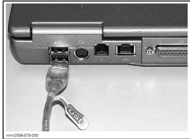
MPI-2 INTERFACE CARD CONNECTED TO USB PORT
