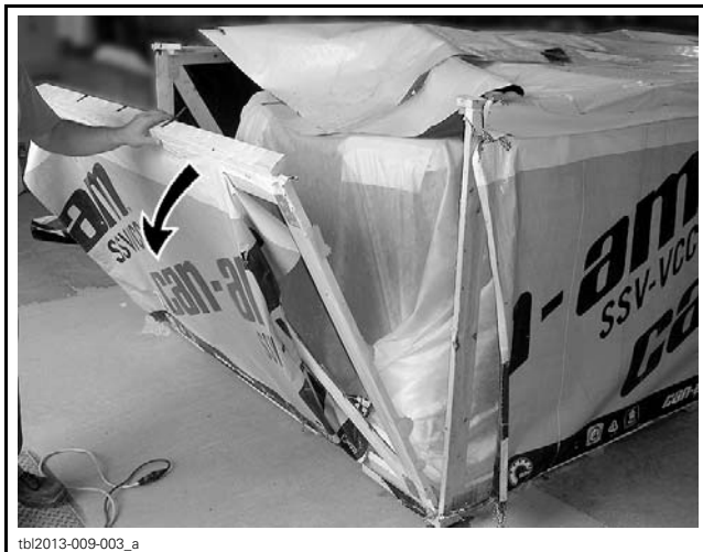
tbi2013-009-003_a PULLING OUT REAR END COVER
