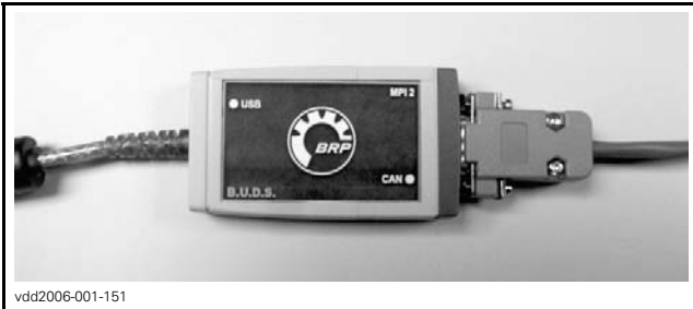
DIAGNOSTIC CABLE CONNECTED TO MPI-2 INTERFACE CARD
