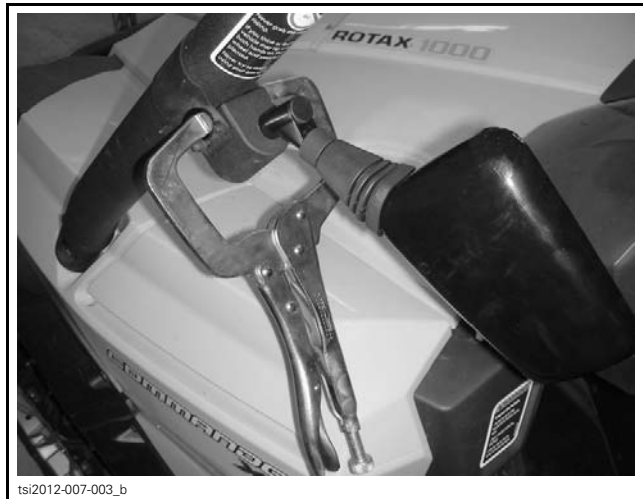
TIGHTENED MIRROR BUSHING INTO MIRROR COLLAR
