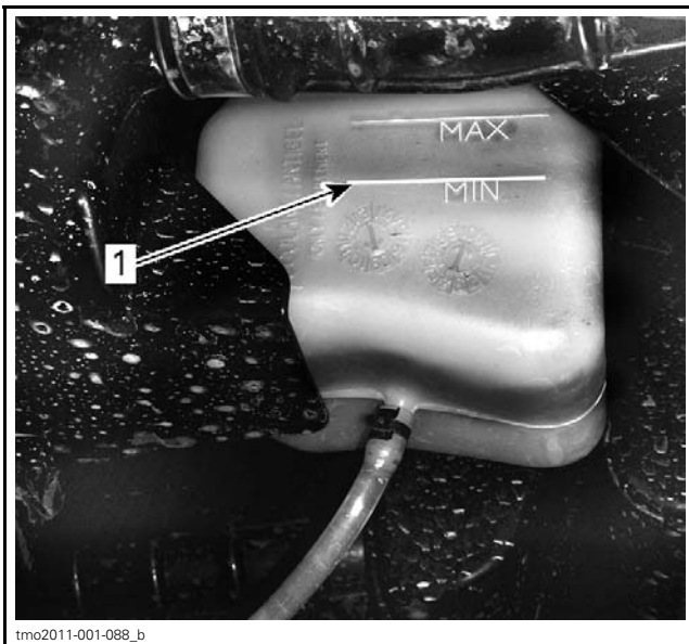
COOLANT EXPANSION TANK 1. MIN level
