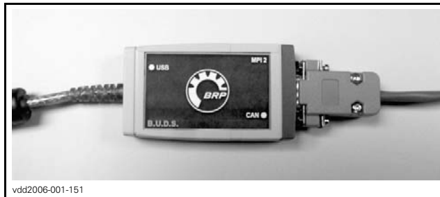
DIAGNOSTIC CABLE CONNECTED TO MPI-2 INTERFACE CARD
