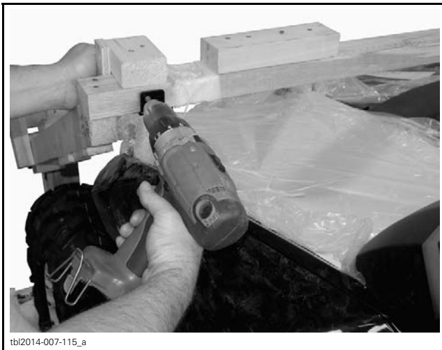
REMOVING SCREWS LOCATED AT REAR OF SUB-CRATE
