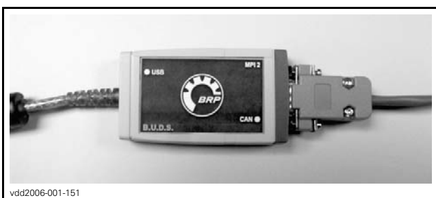
DIAGNOSTIC CABLE CONNECTED TO MPI-2 INTERFACE CARD
