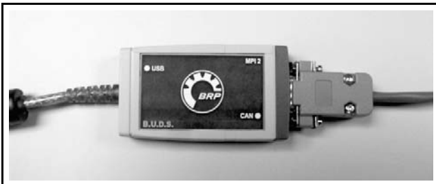
DIAGNOSTIC CABLE CONNECTED TO MPI-2 INTERFACE CARD
