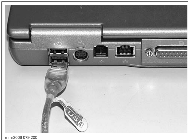
MPI-2 INTERFACE CARD CONNECTED TO USB PORT
