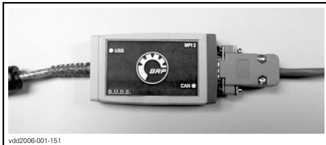
DIAGNOSTIC CABLE CONNECTED TO MPI-2 INTERFACE CARD
