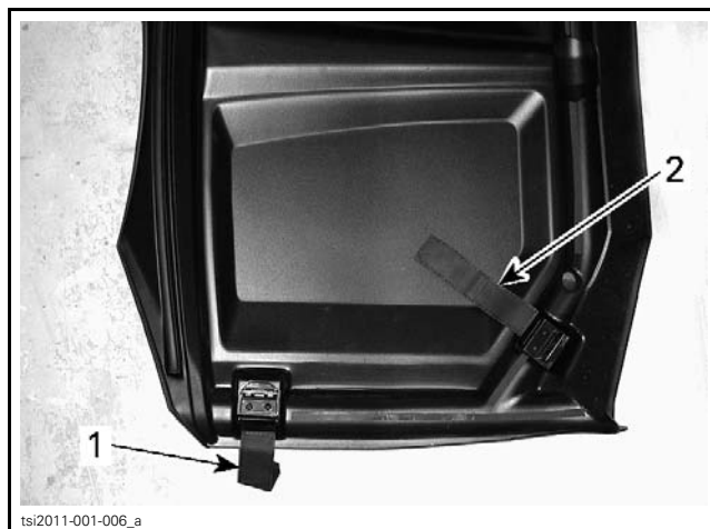
1. Strap toward outside for rear section 2. Strap toward inside for front section
