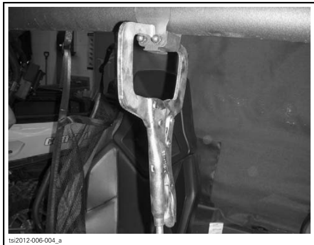
TIGHTENED CENTRAL MIRROR COLLAR ONTO CENTRAL MIRROR BUSHING USING CLAMP PLIERS
