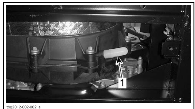
tbg2012-002-002_a 1. CVT drain plug to be removed
