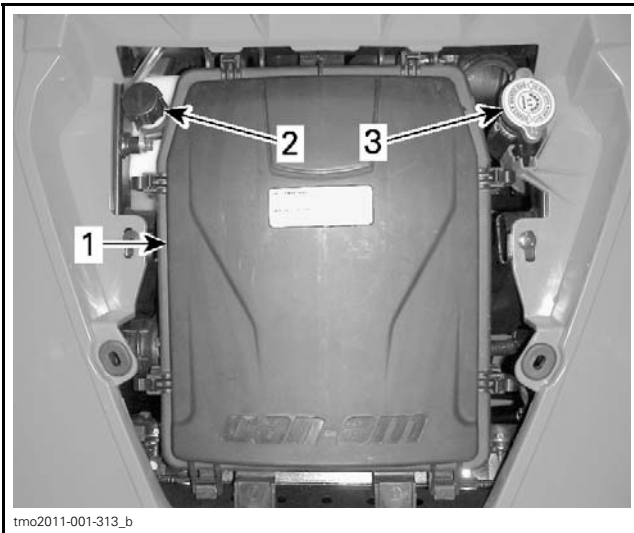
1. Air filter housing cover 2. Coolant expansion tank cap 3. Pressure cap
