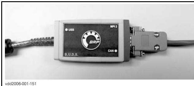
DIAGNOSTIC CABLE CONNECTED TO MPI-2 INTERFACE CARD
