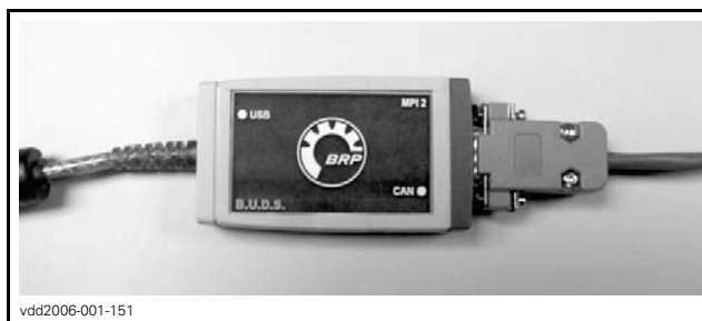
DIAGNOSTIC CABLE CONNECTED TO MPI-2 INTERFACE CARD
