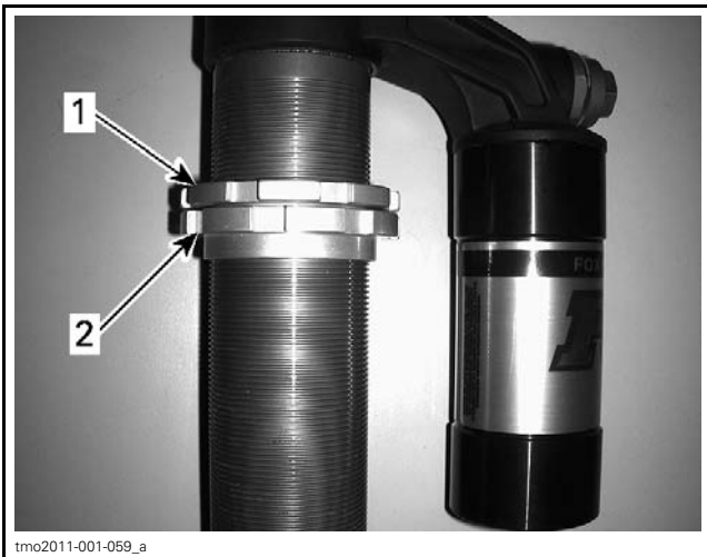
TYPICAL - SPRING NOT SHOWN 1. Loosen top lock ring 2. Turn adjuster ring accordingly
