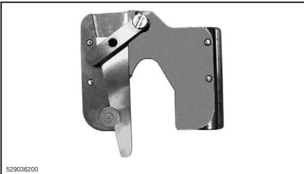
**NOTE:** Align tube of camshaft adjustment tool properly with machined radius on cylinder head.
