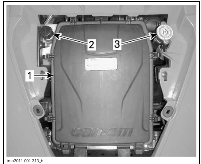
1. Air filter housing cover 2. Coolant reservoir cap 3. Radiator cap
