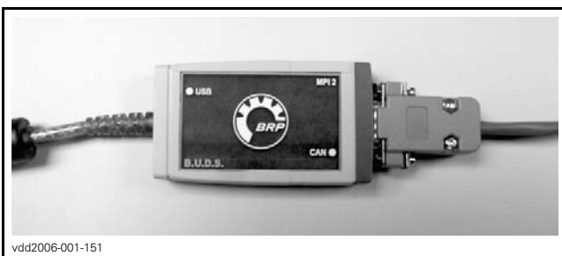
DIAGNOSTIC CABLE CONNECTED TO MPI-2 INTERFACE CARD
