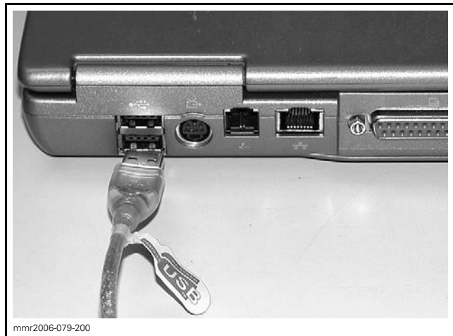
MPI-2 INTERFACE CARD CONNECTED TO USB PORT
