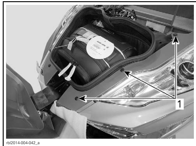
LOW BEAM HEADLIGHT TRIM PANEL ILLUSTRATED (CE MODEL) 1. Plastic rivets to remove (3)
