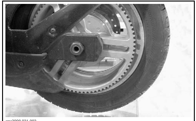
rmr2008-031-003 TYPICAL - SWING ARM ALIGNS WITH A SPOKE
