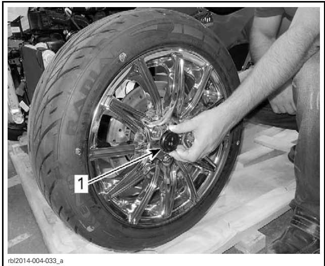
1. Front wheel cap to install, one each side
