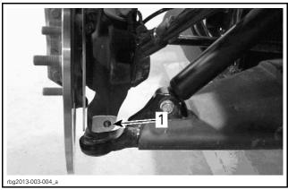
1. Ball joint retaining bolt location
