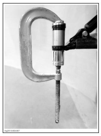
7.3 Tighten C-clamp and press the ball joint into lower suspension arm.
