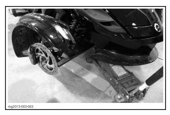
4. Remove the lower ball joint retaining bolt and discard elastic nut.
