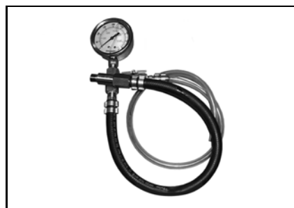
Oil pressure gauge P/N 529 036 142 Mandatory 991 Used for SE5 transmission
