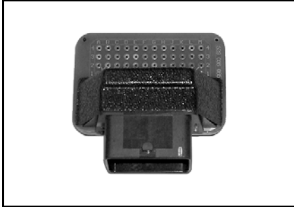
ECM adapter tool P/N 529 036 166 Mandatory ECM BOSCH
