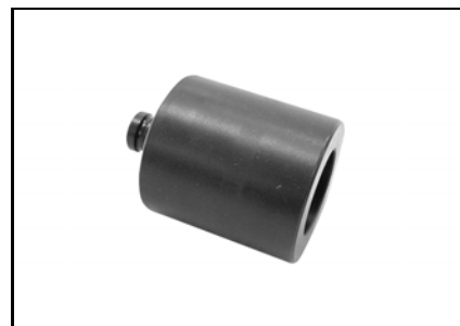
Main shaft seal installer
