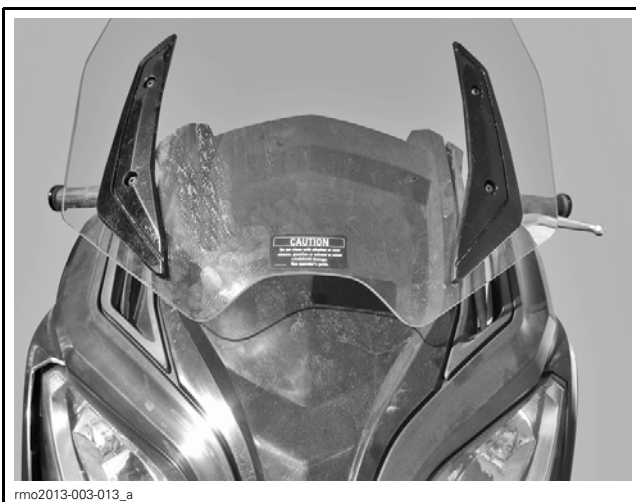
3. Torque windshield retaining nuts.
