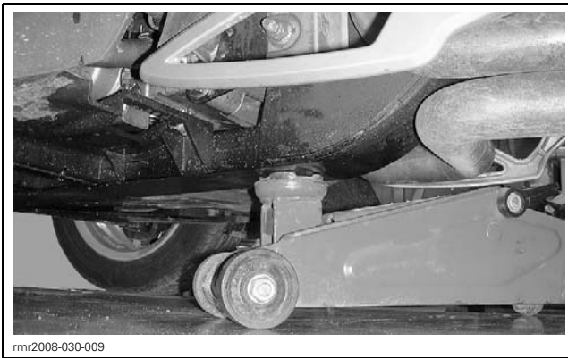
rnr2008-030-009 TYPICAL - LIFT BY THE FRAME
