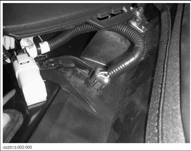
rbi2013-002-005 DLC CABLE INSERTION
