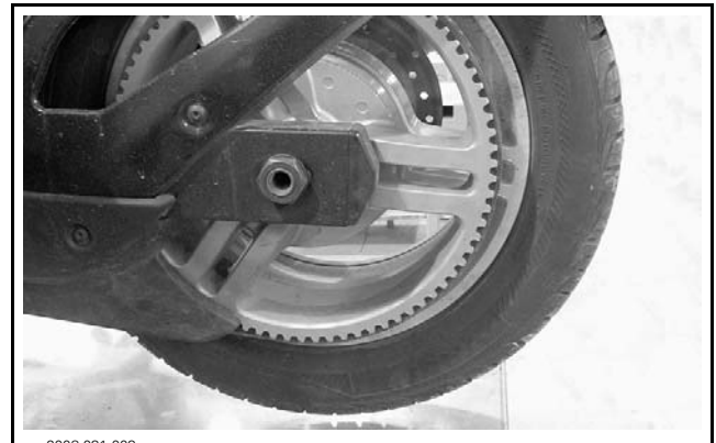
TYPICAL - SWING ARM ALIGNS WITH A SPOKE
