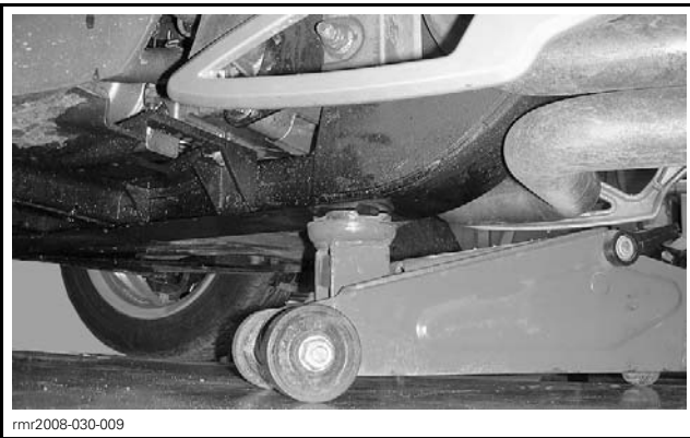
TYPICAL - LIFT BY THE FRAME
