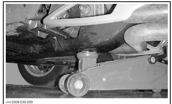
TYPICAL - LIFT BY THE FRAME
