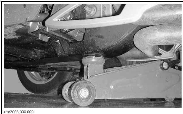
TYPICAL - LIFT BY THE FRAME
