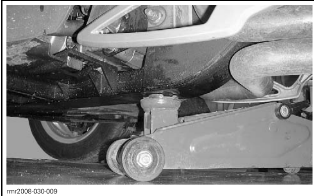
TYPICAL - LIFT BY THE FRAME
