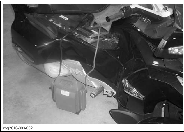
PORTABLE POWER PACK OR A 2 AMP BATTERY CHARGER
