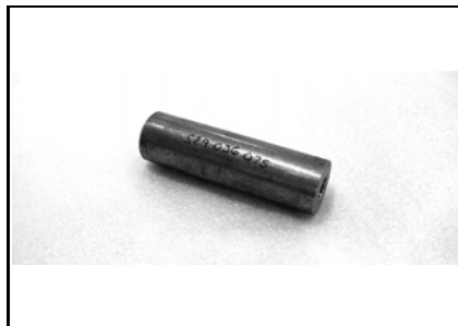
Valve guide installer (6 mm) P/N 529 036 075 Recommended 449, 991 engines Valve guide insertion jig
